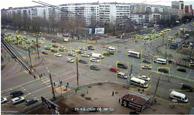
Fig. 4. Example of neural network operation for car recognition
